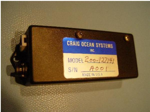
This is a single channel (non-isolated) amplifier, designed to interface to temperature probes, etc. The Line Amplifier provides a precision regulated signal excitation source (5 VDC, for excitation of thermistor temperature sensors).
