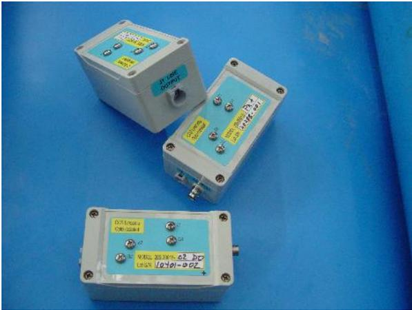
COS Frequency converter, with 3 1/2 digit LCD display and gain and offset adjustments.
