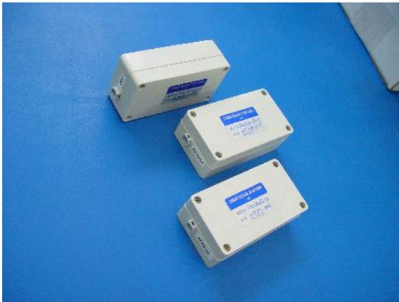
These line amplifiers are designed to interface with 4-20 mA sensors (such as the Conductivity probe). They provide the loop power for the sensor, and convert the sensor output to a standard 0-5VDC signal for direct input to the MCU. These are typically located in the Expander box. DIN rail mounting available.
